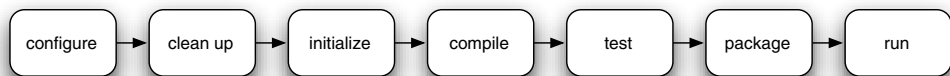
Figure 15.2 Steps for building and running a (web) application. This is a general process for any build of any program. Using Ant or Maven as our build system automates most of these steps.
